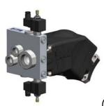
The BY-PASS valve is used together with TWIN FLOW Bent Axis pump. The BY-PASS valve partially reduces, for each pressure output, the pump's oil flow to avoid overheating the system. The BY-PASS valve is composed of an aluminium body mounted on the rear body of the pump fixed by 3 pressure and suction fittings, which works as a screw, 2 normally opened solenoid valves which pilots 2 internal spools.
